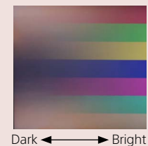
LCD Poor colour reproduction in dark scene conditions
